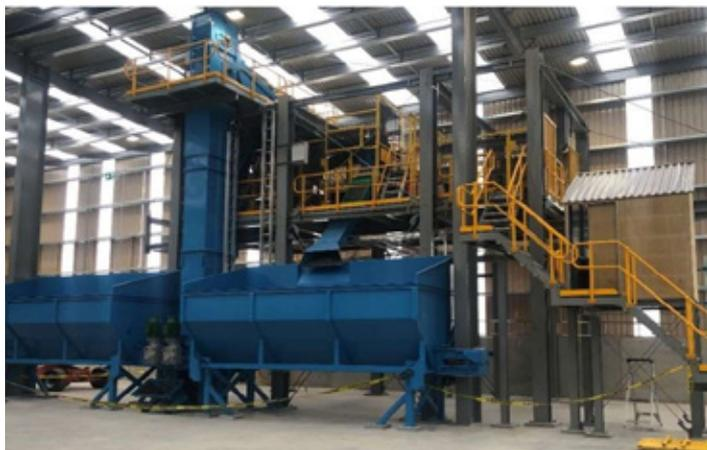
Our client developed a greenfield store for the storage and dispatch of fertiliser to its shareholders. We fabricated, installed, and commissioned blending hoppers, a bucket elevator screen, lump breaker, belt conveyors, structural steel, and chutes.
